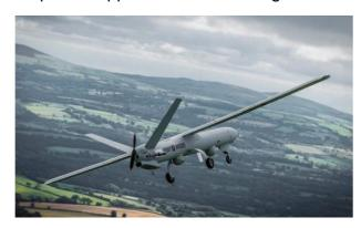
WK has a 36ft wingspan and is 21ft in length. It is powered by a single Wankel engine and can operate up to 16,000ft. It is certified to fly in UK airspace and is flown exclusively by 47th Regiment Royal Artillery. Currently, as a Beyond Visual Line of Sight (BVLOS) controlled aircraft, WK must be operated within segregated airspace which is satisfied by flying within notified Danger Areas.
